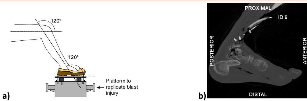
Figure 2: (a) Of the seated postures tested, the one with knee and ankle joints both at 120° was found to cause the most severe type of injury. (b) Sagittal view from a CT scan of an injured specimen tested in this posture.
