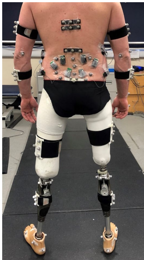
Figure 18: Image showing an amputee with the marker set for investigating the mechanical factors that could be affecting low back pain during activities of daily living.
