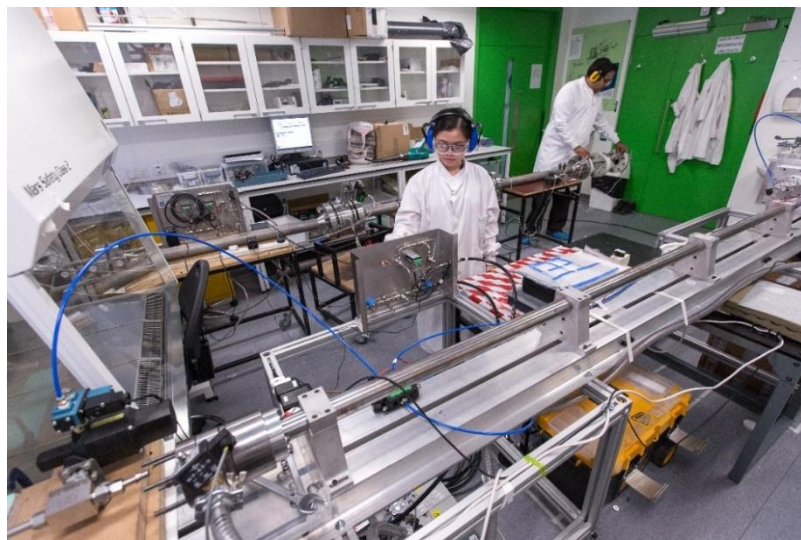
Figure 2: CBIS researchers (foreground) Thuy-Tien Nguyen working with the new compressed-air-driven gas gun system and (background) Hari Arora working with the existing shock tube.
