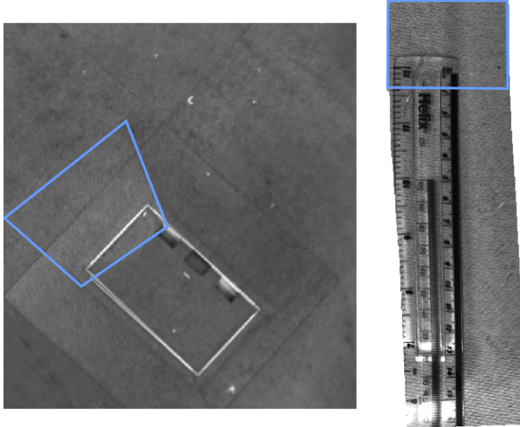
Figure 8: Consistent planar mosaics created by simple stitching of frames using the homographies estimated by our visual odometry system. The field of view of a single camera frame is superimposed for comparison.
