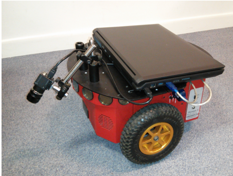
Figure 5: Robot Pioneer 3 DX used for most of the experiments.
