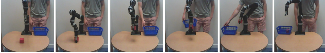
Figure 5: A sequence of images showing the networks ability to generalise. Whilst standing in the view of the camera, it is able to grasp the cube and proceed to the basket. As the arm progresses towards the basket, we move the basket to the other side of the arm. Despite this disruption, the network alters its course and proceeds to the new location. The network has never seen humans, moving baskets, or this table.
