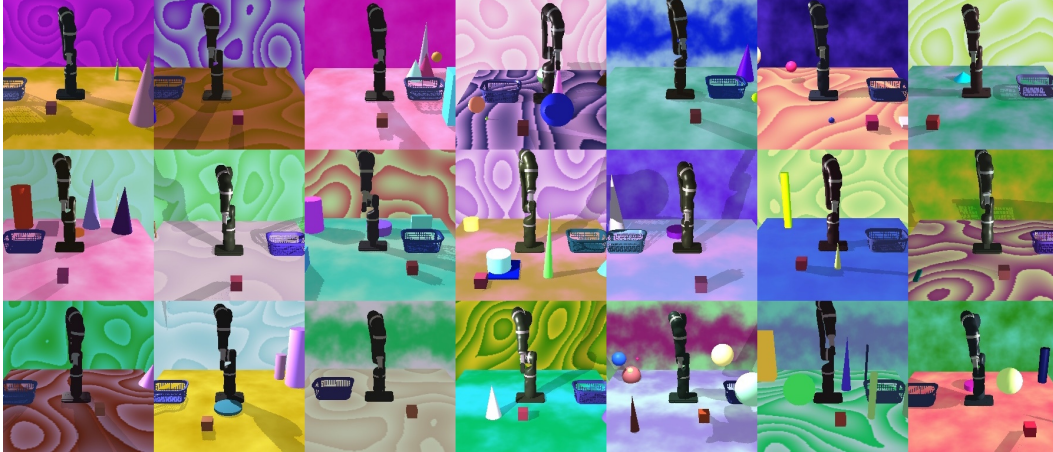
Figure 2: A collection of generated environments as part of our domain randomisation method.
