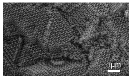
SEM image of "free-standing" 3-DOM material formed from TiO 2 .
