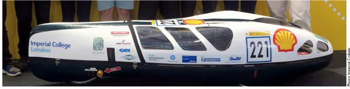
Imperial Racing Green's Shell Eco-Marathon (SEM) team currently competes in the Prototype Hydrogen class of Shell Eco-Marathon. For the 2016/17 they entered the car ICHV01. The car is a hydrogen fuel cell/supercapacitor hybrid vehicle: Fuel cell – H-200 Horizon stack, 200W nominal output; Supercapacitor bank – 18 x 100F capacitors, total 5.5kJ of energy; Motor – Maxon RE 50 24V 200W; Chain drive.
