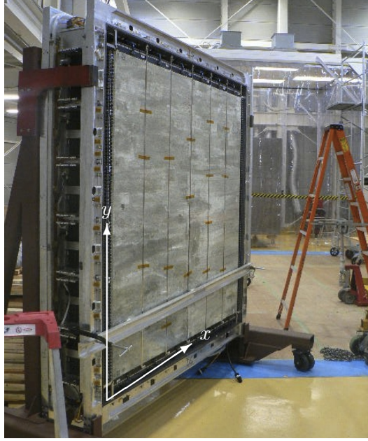
Figure 2.13: The upstream FGD1 detector held in a storage cart prior to installation in the pit. The x - y plane corresponding to the orientation of the XY-modules is superimposed. In an x layer the bars are oriented in the y direction and vice versa. When installed inside the tracker the XY-modules hang down perpendicular to the beam direction [30].
