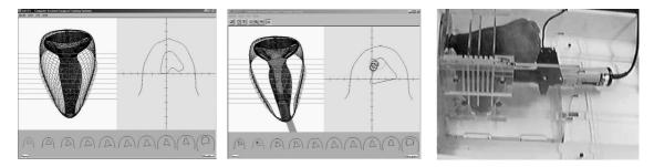
Since the Limbs & Things phantom is opaque to ultrasound, alternative phantoms, made of gelatine and an ultrasound scatterer, were developed. The first prototype (below, left) was based on a resection shape from anatomical diagrams. The second prototype (formers and moulds below, centre and right), based on the Limbs & Things phantom, includes anatomical features, thus allowing a laboratory-based assessment of the *in vivo* system, more closely mimicking the actual operation.
