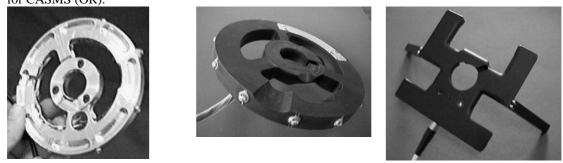
The position of the cutting loop in relation to the resectoscope's sheath is also known. For CASTS, a potentiometer arrangement was attached to the resectoscope (below, left). For CASMS, an alternative sterilisable IRED probe was designed (below, centre).
