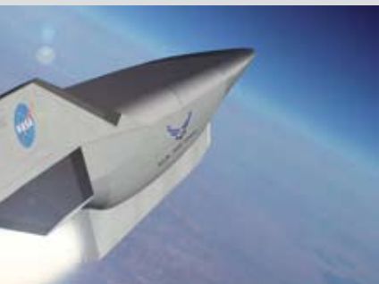
Above: An artist's rendering of the air-breathing, hypersonic X-43C, part of NASA's Hyper-X series of flight demonstrators. NASA will develop, test and fly the Hyper-X series over the next two decades to support development of future-generation reusable launch vehicles and improved access to space.
