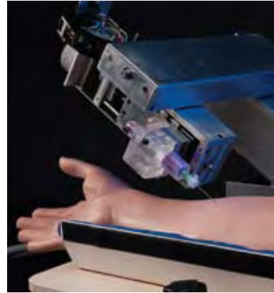
Bloodbot (one of the exhibits at the Hunterian Museum) is a prototype robot for taking blood samples, developed by Dr Alex Zivanovic (Clinical Sciences) and Professor Brian Davies.
