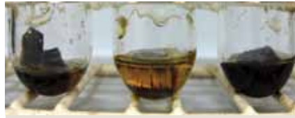
Three different wood samples (Pine, Miscanthus, and Willow) after being treated with ionic liquid.
