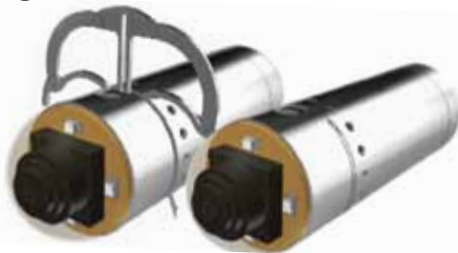
Robotic pill with anchor deployed (left) and retracted (right).
