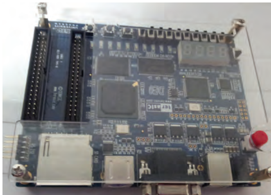
A low cost, small FPGA platform uses very little energy compared to current hardware systems
