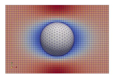
Add forces to fluid Eqs. to impose No-Slip, No-Penetration condition at IB points.
