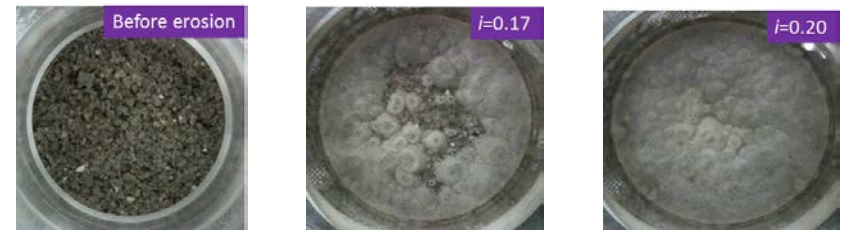
Similar to Skempton & Brogan (1994) on Gap-graded soil (25% fines content; 60% relative density)
