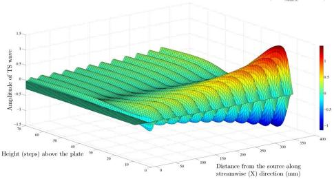
Growing TS wave at 150 Hz sinusoidal excitation from a 2D source ( $Re_{\delta_{l_{source}}} = 875$ )
