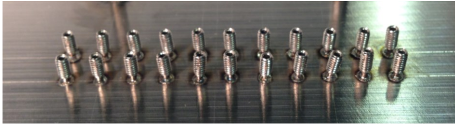
Figure 2.11: A 10 element array of potential drop sensors. Electrodes take the form of grub screws or small diameter dowel pins. For scale the electrode separation is 5 mm in this case.
