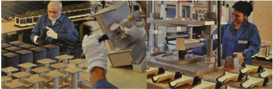
Figure 1.7 Selected stages of TBC blade manufacturing (visual inspection and checks of cooling channels) ( www.alstom.com ).
