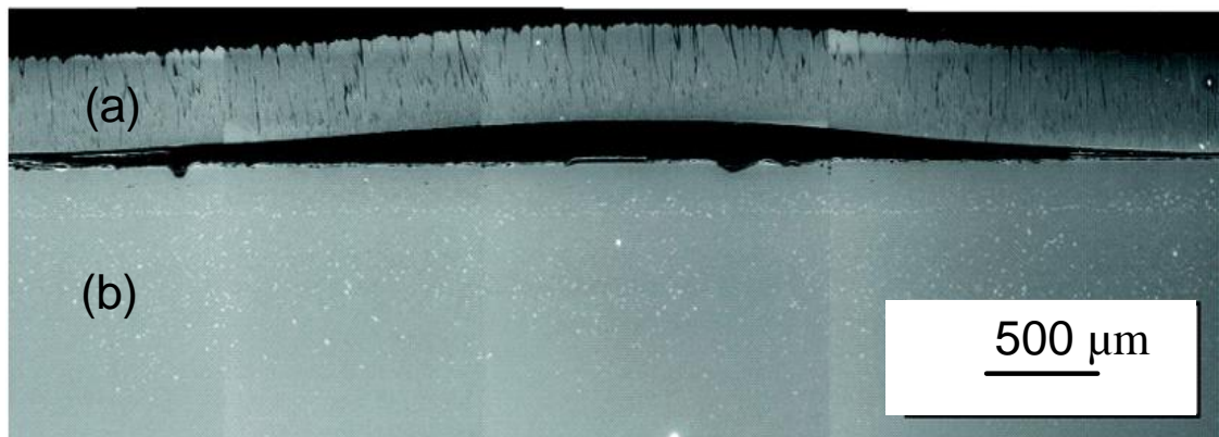
Figure 4.1 Real disbond between ceramic coat and substrate before spalling (Panture et al, 2002) (a) YSZ ceramic coating; (b) BC and nickel super alloy.
