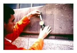
Figure 11. Structural monitoring of cracks with DEMEC Gauge
