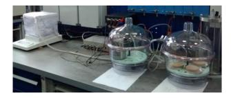
Figure 7. Humidity controlled chambers
