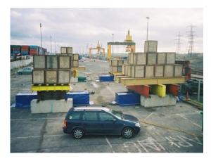
Figure 37. Field monitoring of ground and full-scale pile response to tunnelling in conjunction with Channel Tunnel Rail Link Project (site at Dagenham)
