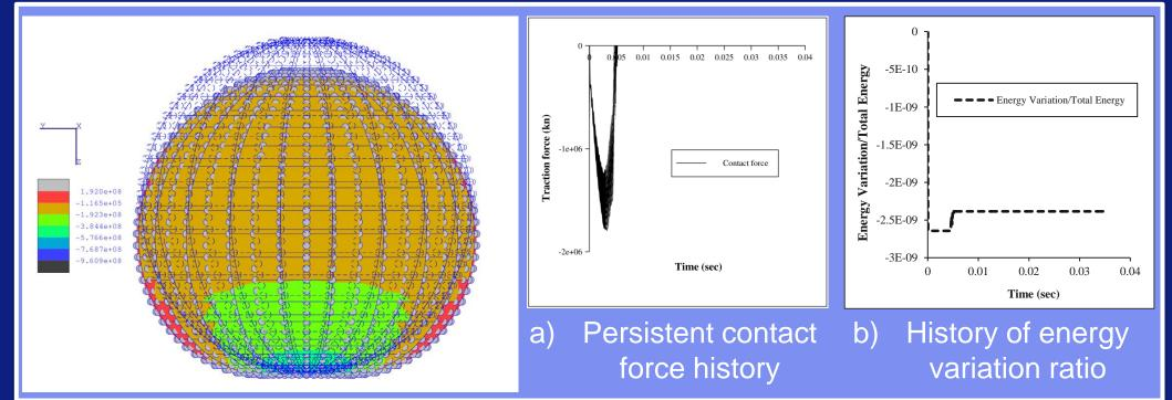
4) Impact of 3D steel cylinder (DVA algorithm)
